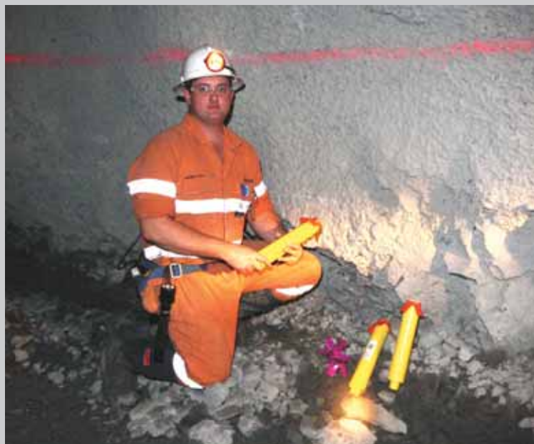
James Lett, Ridgeway Geotechnical Engineer, holds one of the electronic Smart Markers on trial at Telfer and Ridgeway Deeps to give mine planners better insight into ore movement paths and rates.
