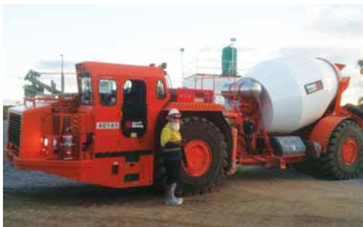
Concrete result: Cement plant operator Charlie Green with Cracow's new agi truck which has been converted from a decommissioned haul truck.
